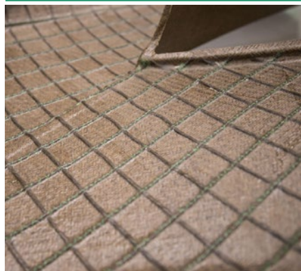
Close-up of the flax composite used in the panels of the Volta Zero
