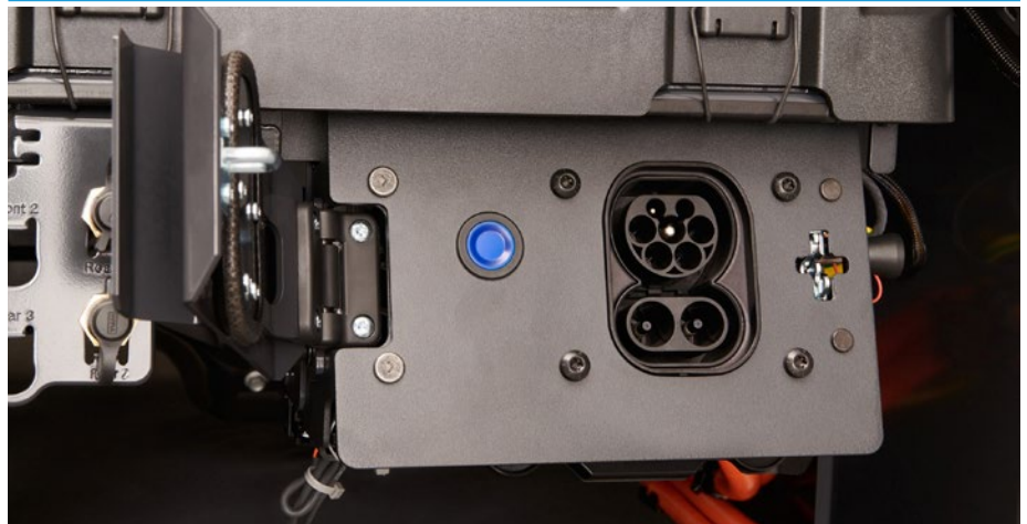
The Combined Charging System connector on Scania's plug-in hybrid
